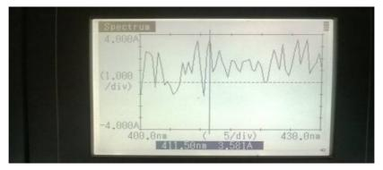
Fig.2. UV-Vis specroscopy Graph obtained for silver nanoparticles synthesized using *P.latifolia* leaves
