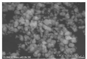
Fig.3. FESEM image of silver nanoparticles synthesized using *P.latifolia* leaves
