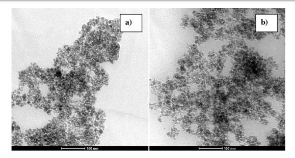
Fig. 1: TEM Images a) Magnetic Iron Nanoparticles (MNPs) b) Chitosan coated MNPs (CNPs)
