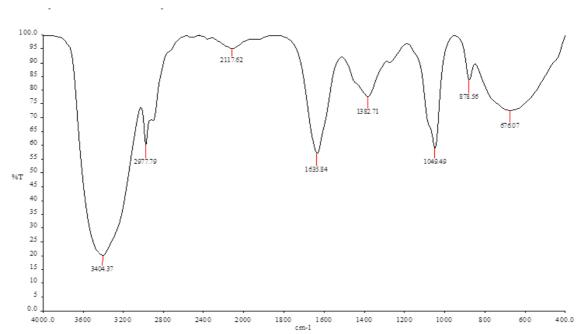
Figure 2: FTIR analysis of silver nanoparticles synthesized using *B.magnifica* leaves
